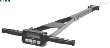
modes of operation: volumetric water content and irrigation management mode. An internal data logger and RS-232 port allow for use with DGPS for georeferenced soil moisture measurements. Rod length without rods is approximately 38". Power: (2) AA alkali batteries, approximately 12-month life (included). Includes software and PC cable. Net wt. 4 lbs, Ship wt. 7 lbs., Ship Dims. 40" L x 15" W x 5" D.
