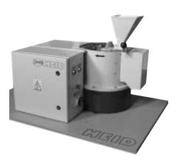
The Model CC is used for coating samples of seed with liquid and powder agents. The unit is equipped with an opening for manual dosing of agents and requires 6 bar (90 PSI) of clean, dry compressed air preventing seed treatment and powders from accumulating beneath the rotor. (Compressor must be obtained locally.)
