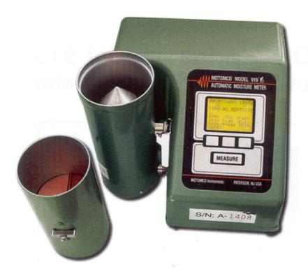
The Model 919® S was designed to perform quick and accurate moisture measurements. For this reason, the operation of the Motomco Model 919® S
